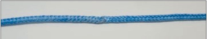
Both ends of the rope are stretched tightly from the splice point outwards - milked out.
