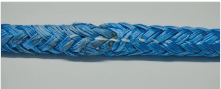
Finished splice. The ends of the rigging twine are knotted and pulled into the rope.
