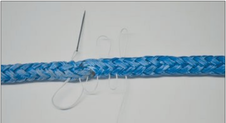
The splices are secured against unintentional loosening by sewing them in a wavy pattern.
